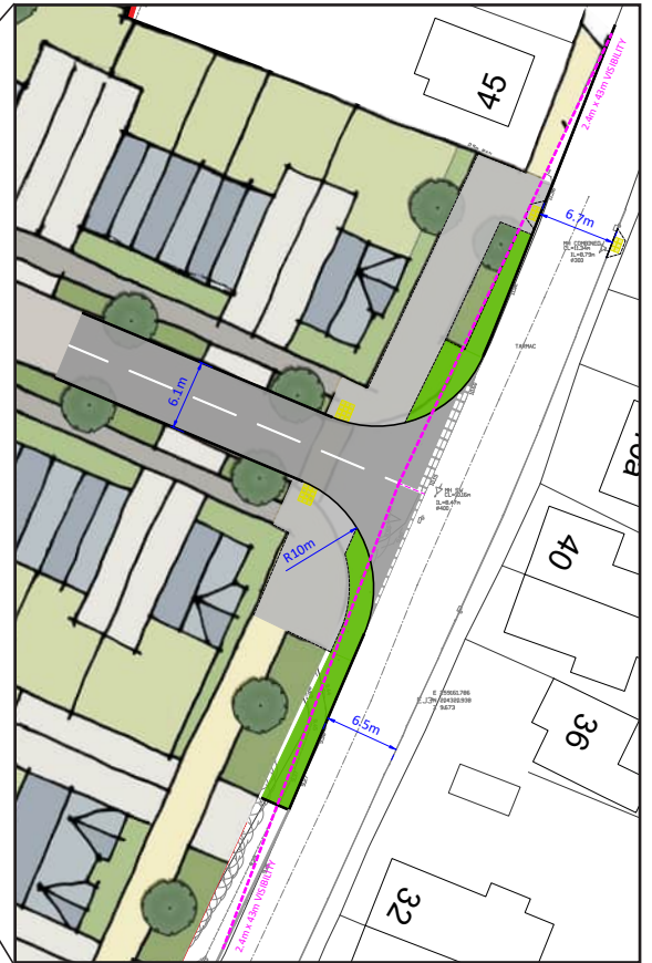
Northern Access: A secondary access point provided onto Woodville Street from the eastern boundary of the site.
