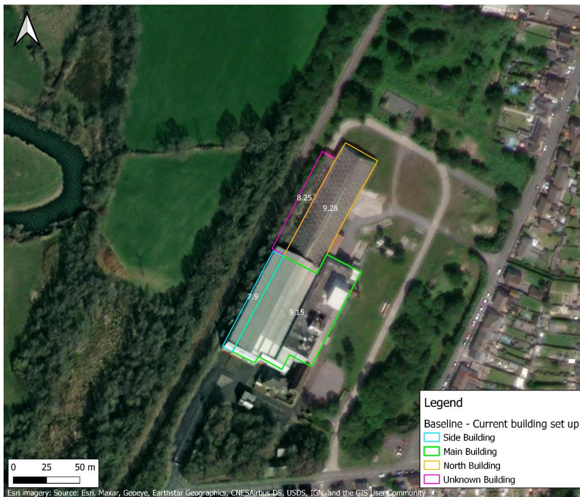
Figure 2-2 - Baseline model set up with building FFL's
